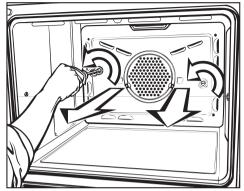
Loosen the screws in the back panel and take it out.
